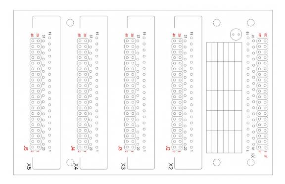
J1-J5 are OEM pin-header locations, and appear immediately next to the DB37 connectors. A 40 pin (2x20) 0.1" spacing header fits the location. OEM pin-header designators are shown in red.
